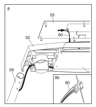
Securely tighten a plastic tie around the Wire Harness (60) and under the indicated hook on the Console (55) to prevent the Wire Harness from slipping. Tighten the plastic tie and cut off the end.
